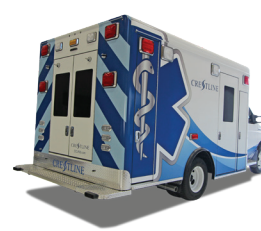
The all aluminum underbody bumper protects the module in low impact collisions.
