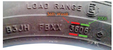
Right: Image showing how to determine age of tires.
